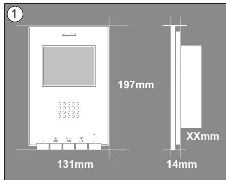
Dimensions of monitor (Height x Width x Depth\*):
