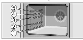
The accessories can be removed halfway until they are secured. This makes it easy to remove food.
